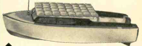
▲ SOLAR-POWERED BOAT uses 40 solar cells to run its small motor, moving majestically through the water under radio control on sunny days. The sun ship was built by the Rev. Robert W. L. Mark of Hawley, Pa., known to RADIO-ELECTRONICS readers as author of articles on the old one-tube Twinplex circuit.
