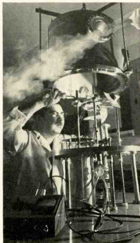
Senior technician Paul Raygor prepares for an experiment in the Westinghouse ultra-high vacuum chamber.
