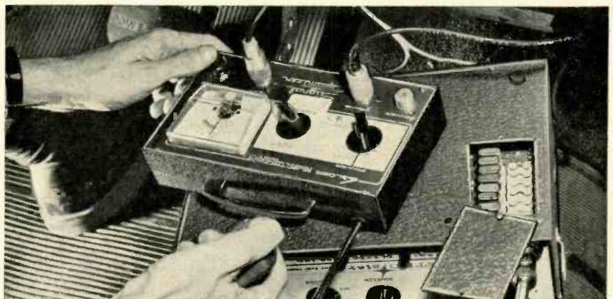
Here, power meter is inserted between transceiver and antenna, as shown in Fig. 4. If transmitter checks OK, trouble is narrowed down to receiver or audio.
