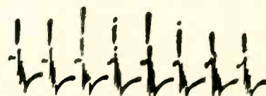
Fig. 3 - Normal parade display shows all cylinders in a row.
